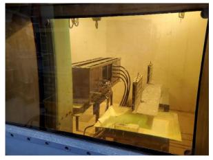
NextGEN RPI Radiation Testing – Passed 750kRads
