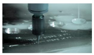
Westinghouse provides precision CNC engraving on a variety of materials.
