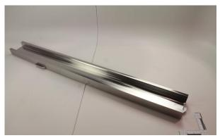
Loop stop isolation valve (LSIV) guide channel machined by Westinghouse
