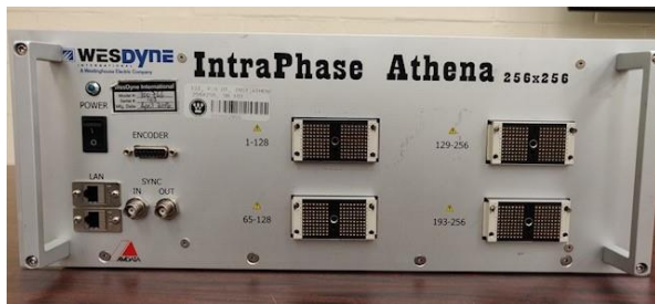
Westinghouse Athena PA System
