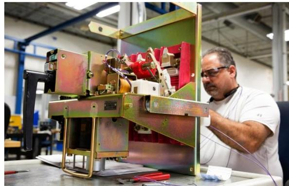
*Westinghouse DB circuit breaker being assembled*
