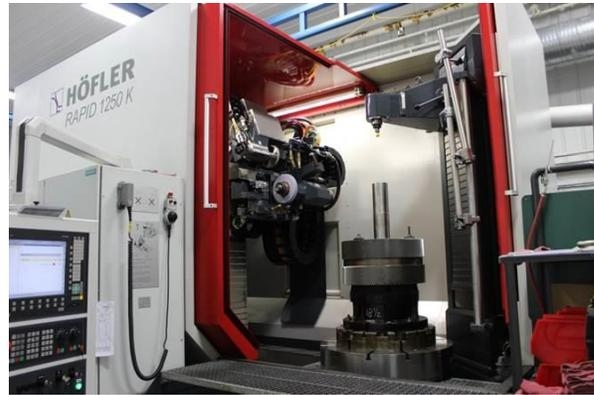
*Westinghouse and Nuttall partner to offer state-of-the-art manufacturing capabilities; pictured is a gear grinder with a typical high-speed gear mounted.*
