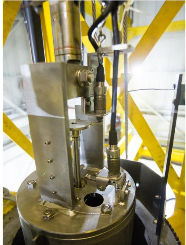
*Gripper actuating cylinder and top mast plate*
