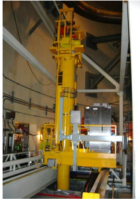
Model WR Controls System with optional trolley installed in U.S. nuclear plant
