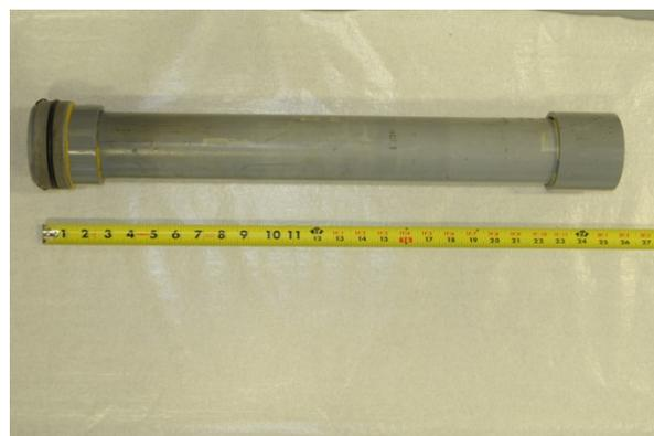
*Typical ion exchange filter*
