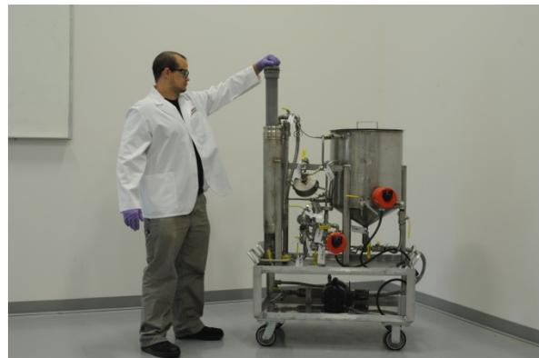
*Operator changing out an ion exchange filter*
