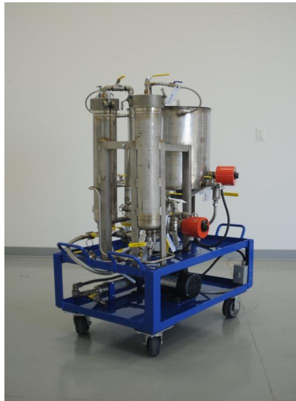
*Mini System Decontamination (MSD) Skid*
