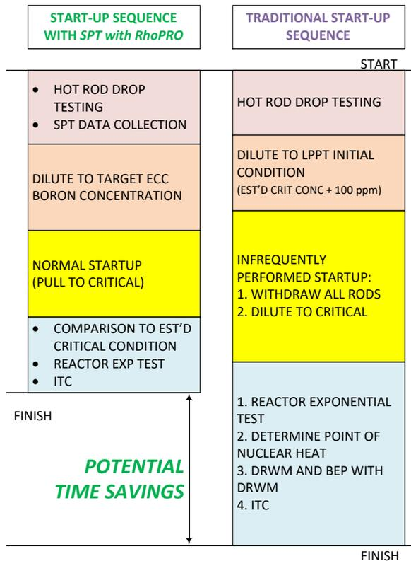
*Traditional LPPT is a direct barrier to MODE 1 entry. SPT with RhoPRO simplifies and streamlines post-refueling startup activities between MODE 3 and MODE 1. As a result, core design verification is almost entirely removed from outage critical path, putting the customer back on the grid faster than ever before.*
