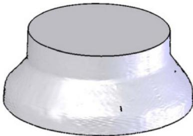
Image of fillet weld and adjacent nozzle part as result of profilometry measurement
