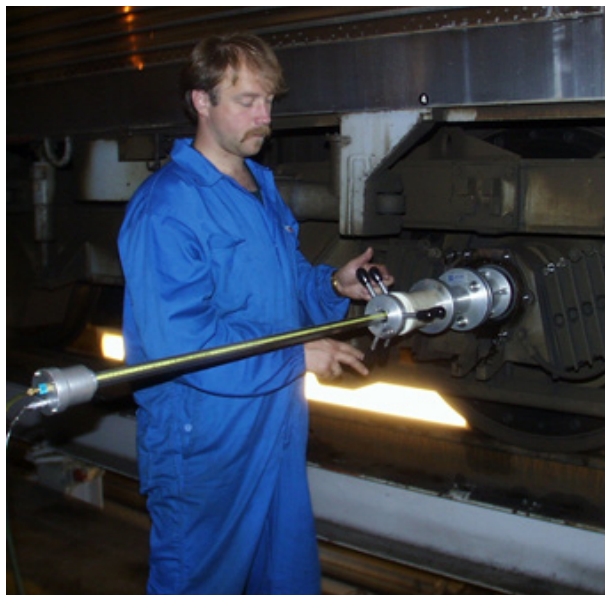
Current semi-automated inspection of train axle using WesDyne equipment
