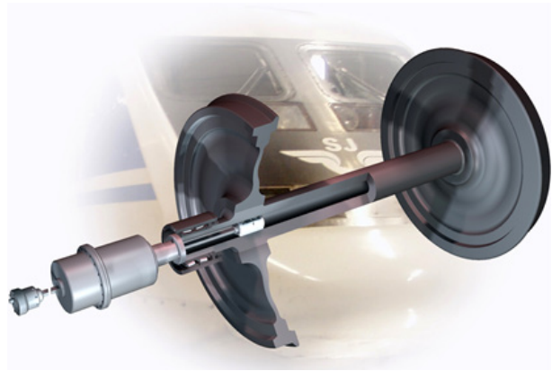
Automated AxMan inspection system for train axles
