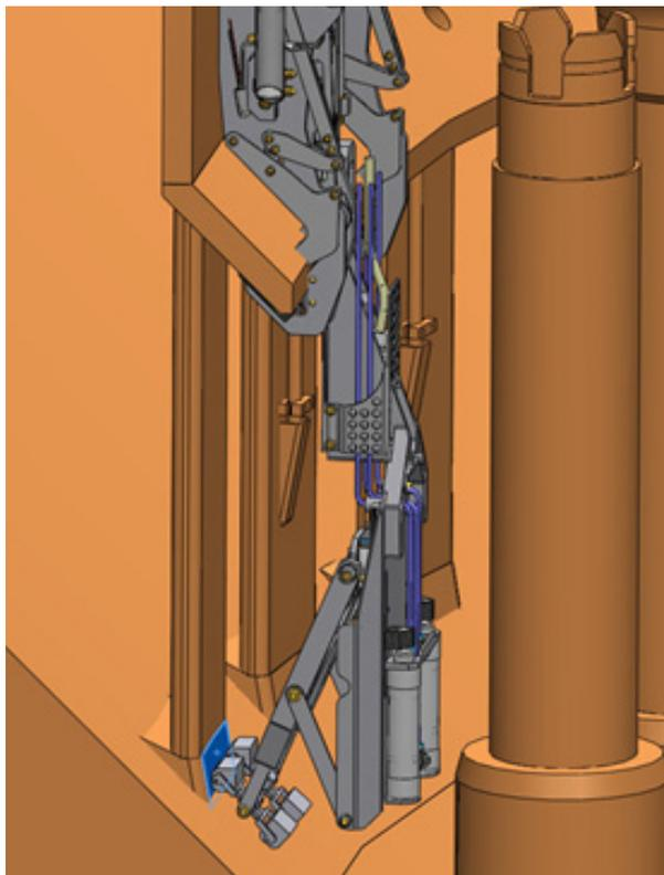
Configuration for sizing of defect using time-of-flight diffraction (TOFD)
