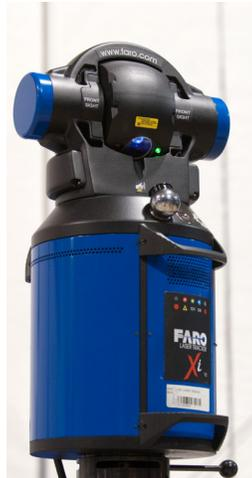
Laser tracking interferometer
