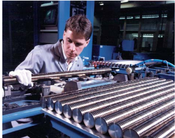
Uranium metal fuel rods machined before insertion into Magnox cans
