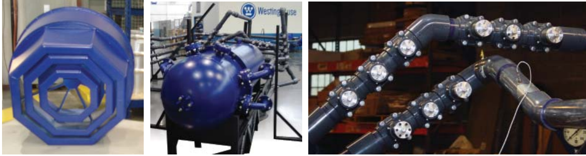
BWR steam dryer qualification for power uprates includes acoustic load predictions, evaluation of structural responses to various combinations of loads, and real-time power ascension analysis and monitoring, among other items. In these photos, a scale model of the the steam dryer and the entire steam delivery system are used to predict acoustic vibrations at extended power uprate conditions.
