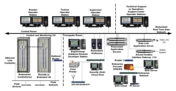
Typical Plant Process Computer System Architecture
