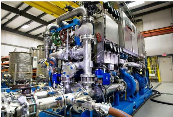
*Westinghouse has developed a variety of chemical decontamination processes and skid-mounted equipment, such as that shown above which is capable of processing system volumes greater than 25,000 gallons.*
