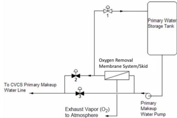
Figure 2: Fuel Burnup Boron Dilution Standby Alignment
