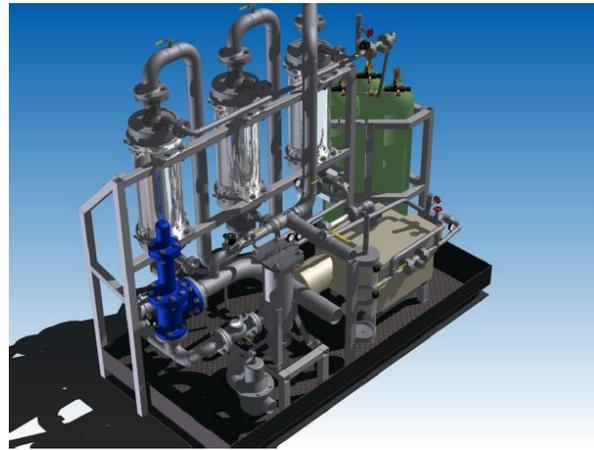
Figure 1: MARS Skid Rendition of Preliminary Design
