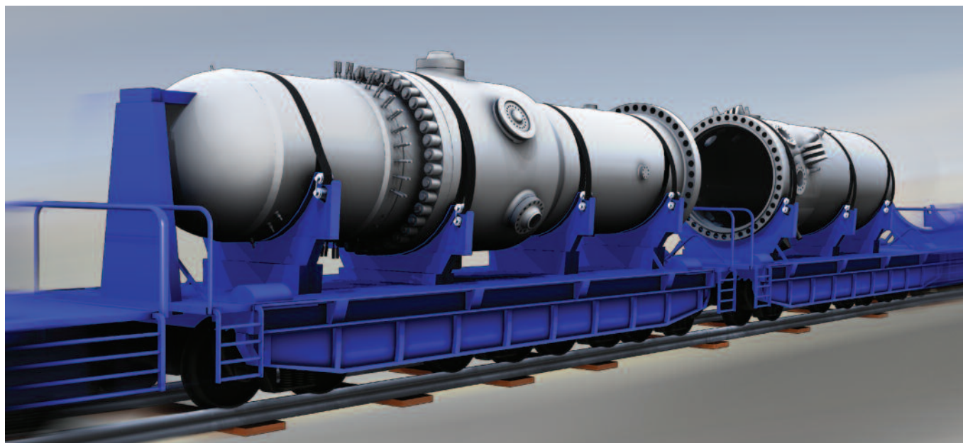
Concept art illustrating rail shipment of the Westinghouse SMR integral reactor pressure vessel. Module shipment size configurations can be adjusted to the preferred form of transportation to a particular site.
