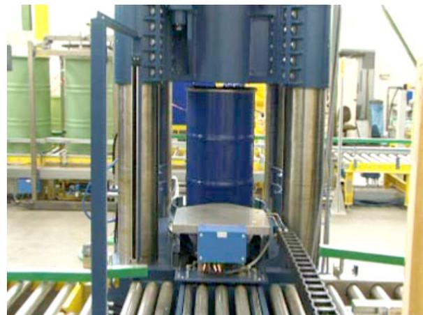
Supercompactor with delivered crumble drum of radioactive waste
