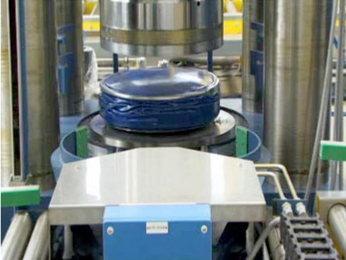
Crumble drum after compaction
