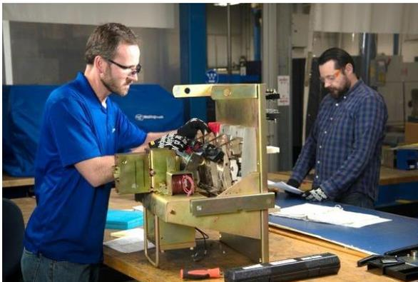
*Original DB circuit breaker in reassembly*
