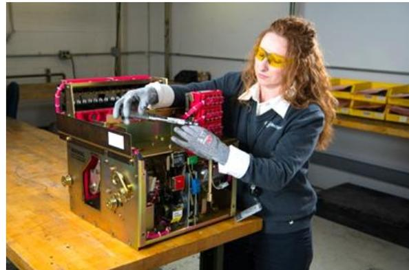
*Original DS circuit breaker being reassembled*
