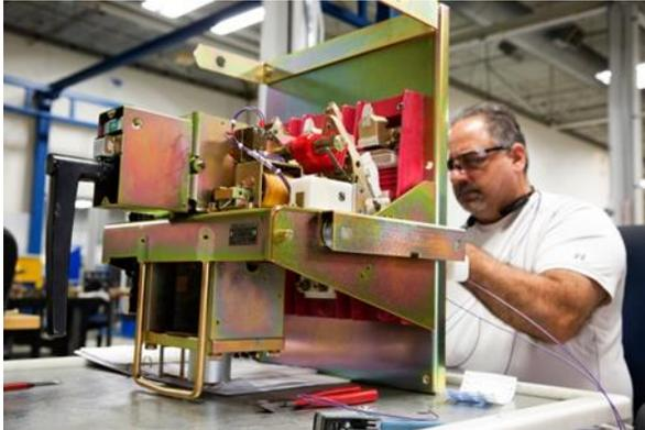
*Original DB circuit breaker being reassembled*
