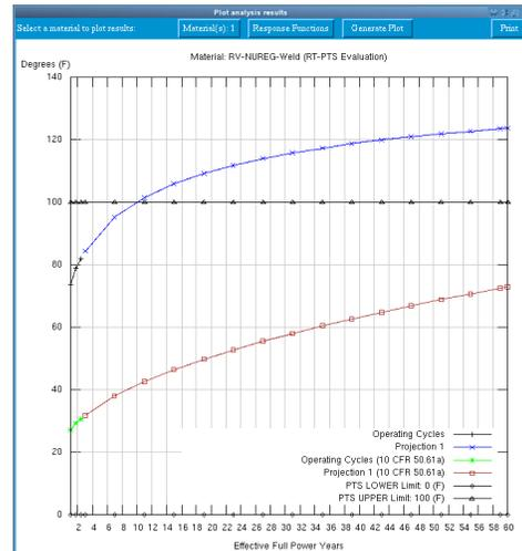
RT<sub>PTS</sub> parameters can be calculated and displayed directly by the RadTrack system
