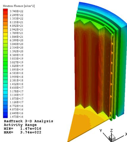
The RadTrack code system generates 3-D contour plots of radiation exposure for the reactor vessel and internals
