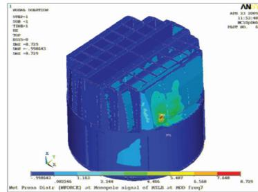
Steam dryer finite element model
