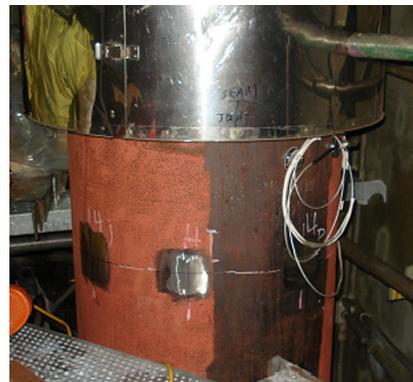
Typical installation of strain gauges on a main steam line
