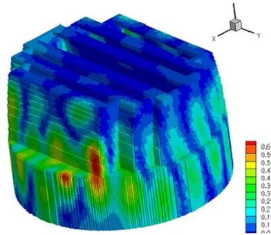
High resolution three-dimensional acoustic pressure field surrounding steam dryer
