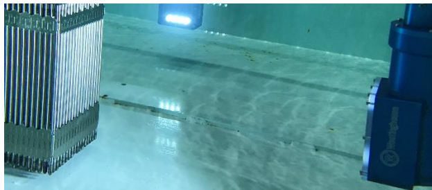
One 5-Sided Camera Viewing Fuel Assembly
