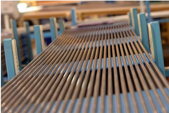
*AXIOM fuel tubing being produced at Westinghouse's Specialty Metals Plant in Blairsville, PA*
