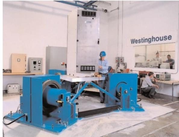
*Westinghouse seismic shake table*
