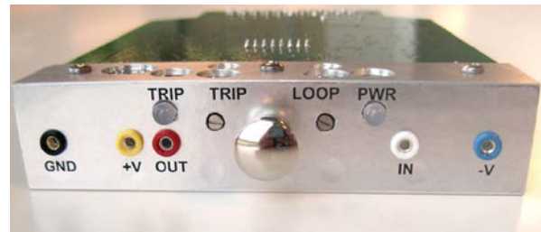
The 10010B94G02 card includes status LEDs that show the present state of the card.
