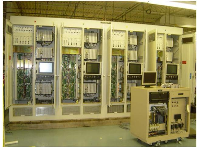
Four-channel core protection calculator system and input/output simulator
