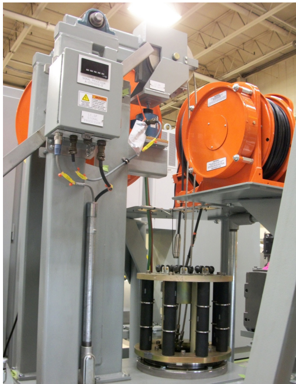
Load-weighting system and cable reels
