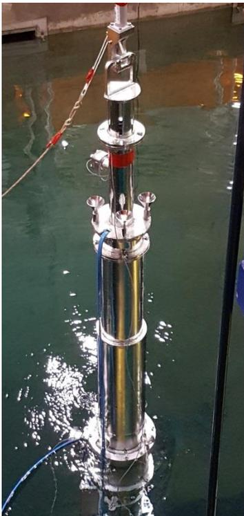
*FAST Equipment is lowered into Spent Fuel Pool*
