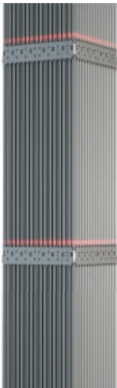
Laser Line on a PWR Fuel Assembly during measuring.
