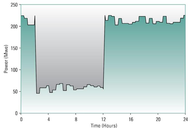
Sample change in power output vs. time during load follow and frequency control
