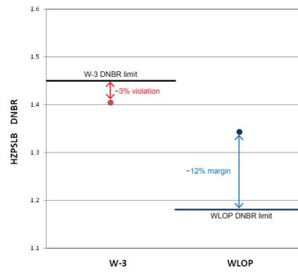
Comparison of DNBR results for hot zero power steamline break
