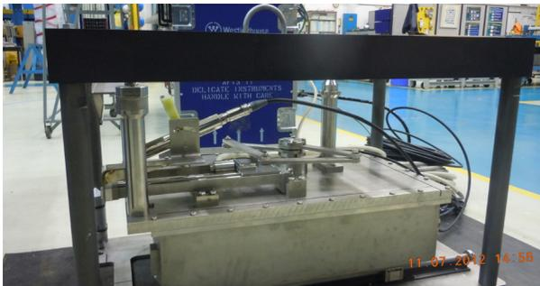
AFIS II manipulator mounted in lift rig
