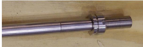
Instrument tube tie rod top with nut
