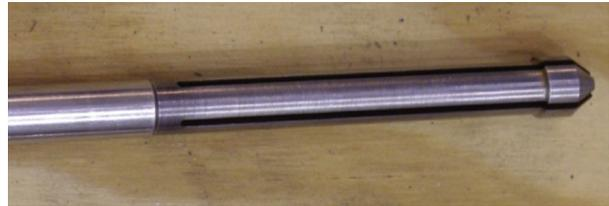
Instrument tube tie rod bottom expansion tip
