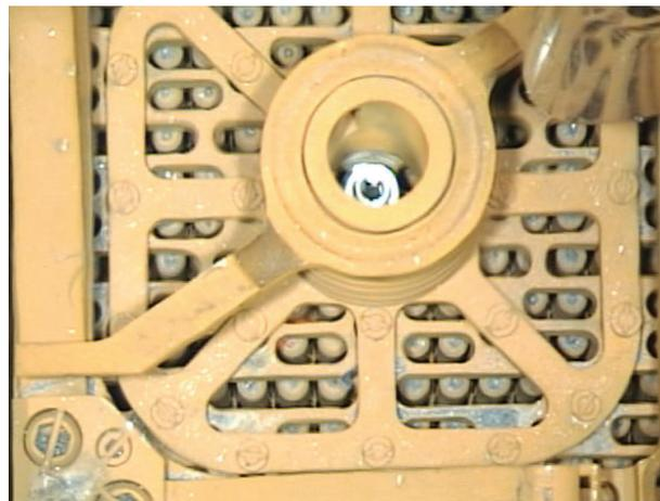
A completed installation with thimble plug assembly installed
