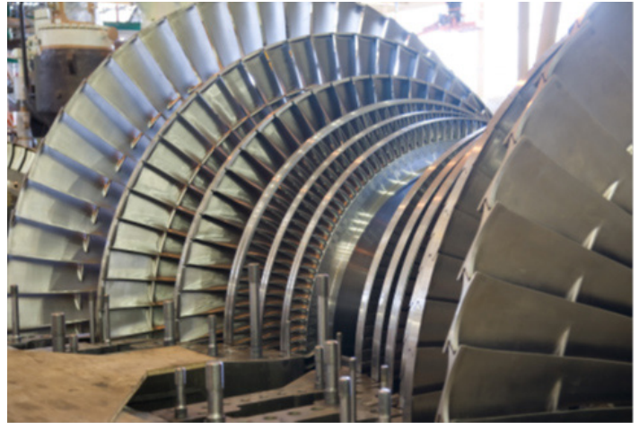
A replacement turbine rotor increases plant electrical output.
