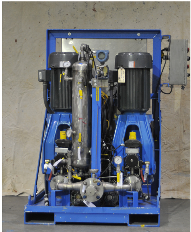
Dual pump skid provides system flow.
