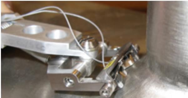
Flexible time of flight diffraction (TOFD) technique probe for curved surface; each footprint less than 3\*3 mm
