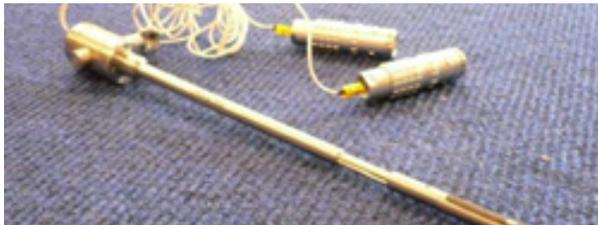
Flexible probe  $\varnothing 5.65$  mm consisting of two pulse echo probes, used for fuel alignment pins inspection
