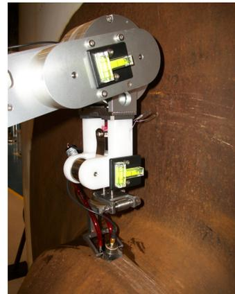
Inner radius arm end-effector scanning the nozzle barrel
