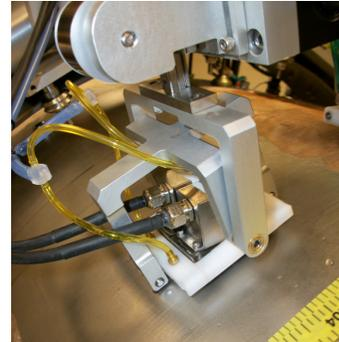
Dissimilar metal scanner with circumferential phased-array probe
