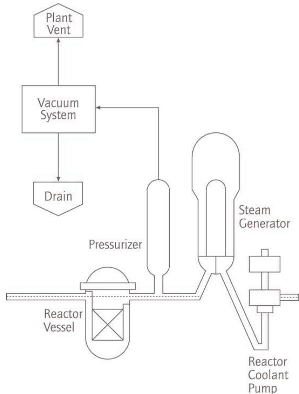
*Illustration of the Reactor Coolant Vacuum Refill System arrangement.*
