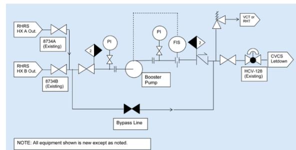
Flow schematic for purification booster pump and associated equipment
