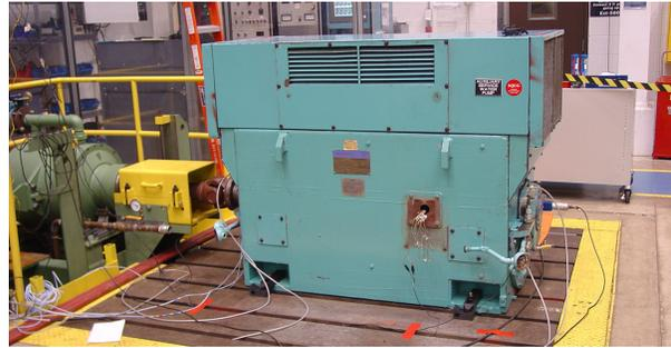
Dyno testing of a 2,000-hp motor
