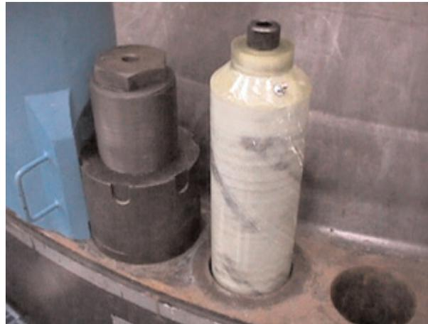
The reactor vessel stud enclosure installed over a stud in the reactor mock-up at Waltz Mill
