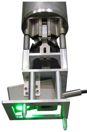
False fuel assembly on refueling machine gripper
