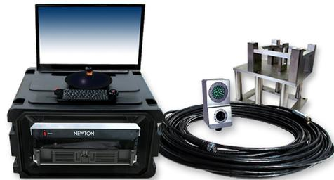
NM200E system hardware includes ruggedized control console, underwater camera with built in LEDs, underwater cable and false fuel assembly.
