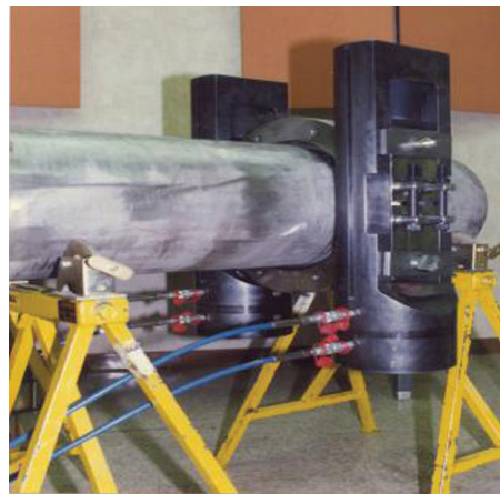
Application of MSIP to 12-inch pipe
