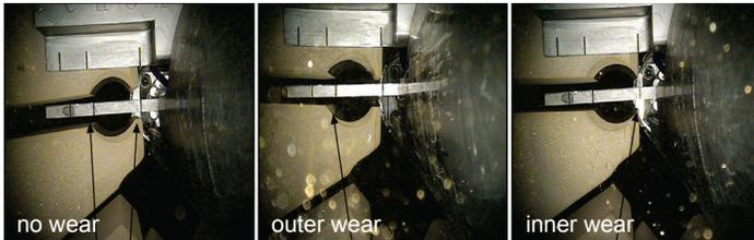
Guide card wear observed during guide card wear measurement
