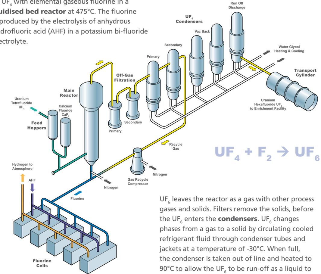
$UF_6$  leaves the reactor as a gas with other process gases and solids. Filters remove the solids, before the  $UF_6$  enters the **condensers**.  $UF_6$  changes phases from a gas to a solid by circulating cooled refrigerant fluid through condenser tubes and jackets at a temperature of -30°C. When full, the condenser is taken out of line and heated to 90°C to allow the  $UF_6$  to be run-off as a liquid to the Hex filling station. Uncondensed gases are recycled back to the reactor.
