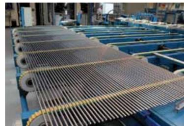
light water reactor fuel top end rod line
