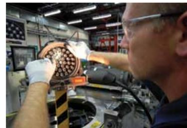
advanced gas-cooled fuel element assembly
