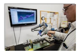
Portable CMM 3D Imaging and Measurement
