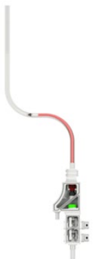
Reactor vessel and leak-off line environment (left) with clamping module and a tool into the pipe (right)
